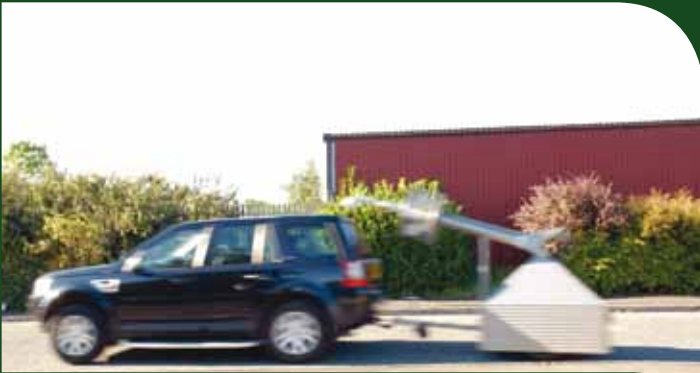
The iGuard tower can be collapsed and towed by a car
